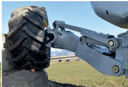
Intelligent arrangement of pivot points
